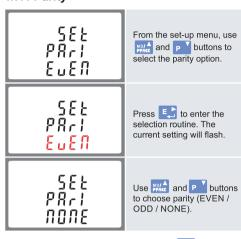
On completion of the entry procedure, press to confirm the setting and press WA to return to the main set up menu.
