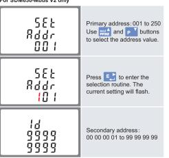
On completion of the entry procedure, press 🔁 to confirm the setting and press V/A to return to the main set up menu.
