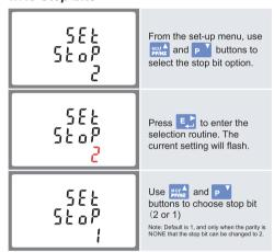
On completion of the entry procedure, press to confirm the setting and press V/A to return to the main set up menu.
