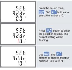
On completion of the entry procedure, press 🛃 button to confirm the setting and press [V/A] button to return the main set-up menu.
