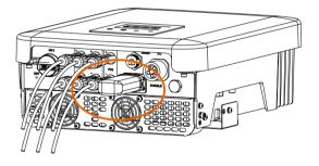
2) Insert U-disk with upgrade package\* into the DONGLE port on the bottom of the inverter. Then turn on DC switch and connect the PV connector, the LCD will show a picture as on the right.
